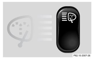
The headlamp washer can be activated with the electronic key in steering lock position 2.
